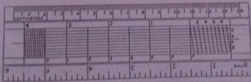
Fig. 1.3 Decimal Diagonal Scale in Inch Units
